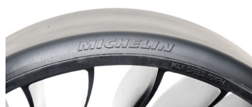
When the "MICHELIN" sidewall lettering is no longer visible due to wear, the caster has reached the end of its ideal life
