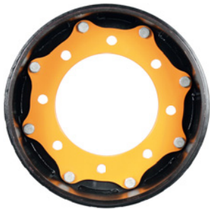
Hub Adapter MSPN 47139 12 mm thick 1015 Carbon Steel / Reversible 8.75" (222.3 mm) Center Dia. 8 x 10.91" Bolt Pattern 0.79" (20 mm) Bolt Holes, No Taper
