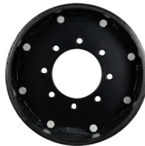
Hub Adapter MSPN 47868 12 mm thick 1015 Carbon Steel / Reversible 6.0" (152.4 mm) Center Dia. 8 x 8.0" Bolt Pattern 0.67" (17 mm) Bolt Holes, Tapered
